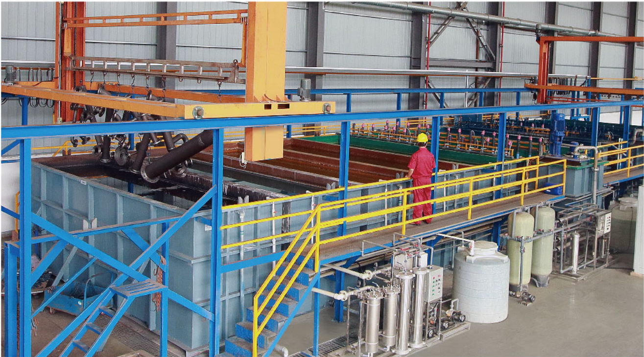
Our capacity to handle 1 single component of 1.5 ton net weight and length up to 2 meters. Electrophoretic coating production line
